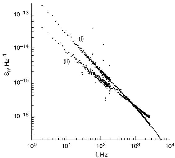
**Fig. 4** Normalised noise power density spectrum after annealing and after 3610 min exposure to bandgap light for n-type ( $10^{-4}$ ) a-Si:H
