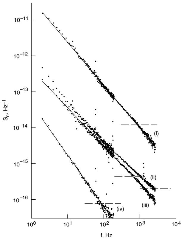
**Fig. 1** Normalised noise power density spectra for four *a-Si:H* samples
