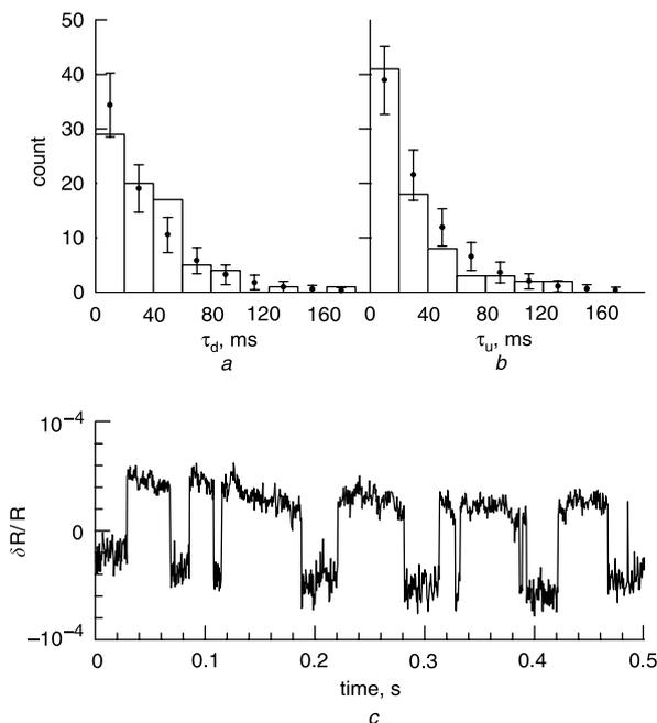
**Fig. 7** Random-telegraph-like noise in n-type a-Si:H
